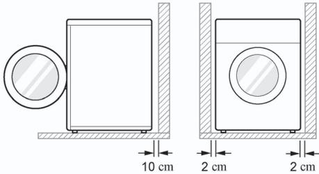
**Level floor :** Allowable slope under the entire washing machine is 1°.
