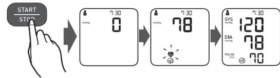
When the [START/STOP] button is pressed, the measurement is taken and saved automatically.
