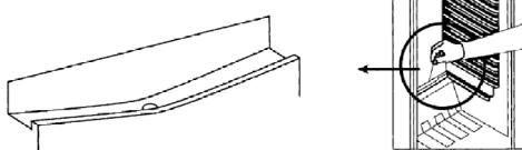
Make sure that the drain gully and the drain opening are not blocked so that the water produced in the refrigerator can always flow off unobstructed.
